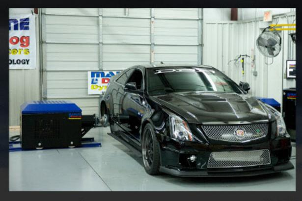
DBR High Performance is the hottest place in Tennessee to get your car dynoed. DBR offers dyno testing, custom tuning, and in-house dyno time rental so you can do your own tuning. Our Mainline Prohub 2000 Dyno allows us to accurately calibrate and dyno 2000+ hp. A hub dyno is very beneficial in the tuning process because there is no danger of the vehicle coming off the dyno. It also has no issues with tire spin which allows us to have very precise calibration, especially on big power cars.
